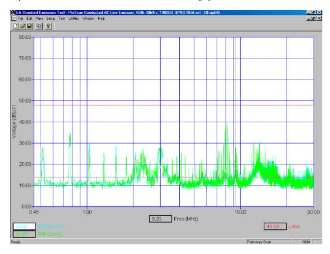
120 volt, 60 Hz ac input to ac Adapter, Globtek, model number SA-052AU-1, part number WR91A2400CCP connected to the GPRS OEM Radio Modem kit, part number PRD-4230-002 in idle mode.
