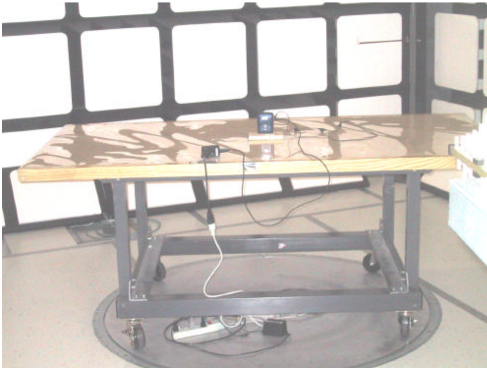
Radiated Emissions at 3.0 metres
