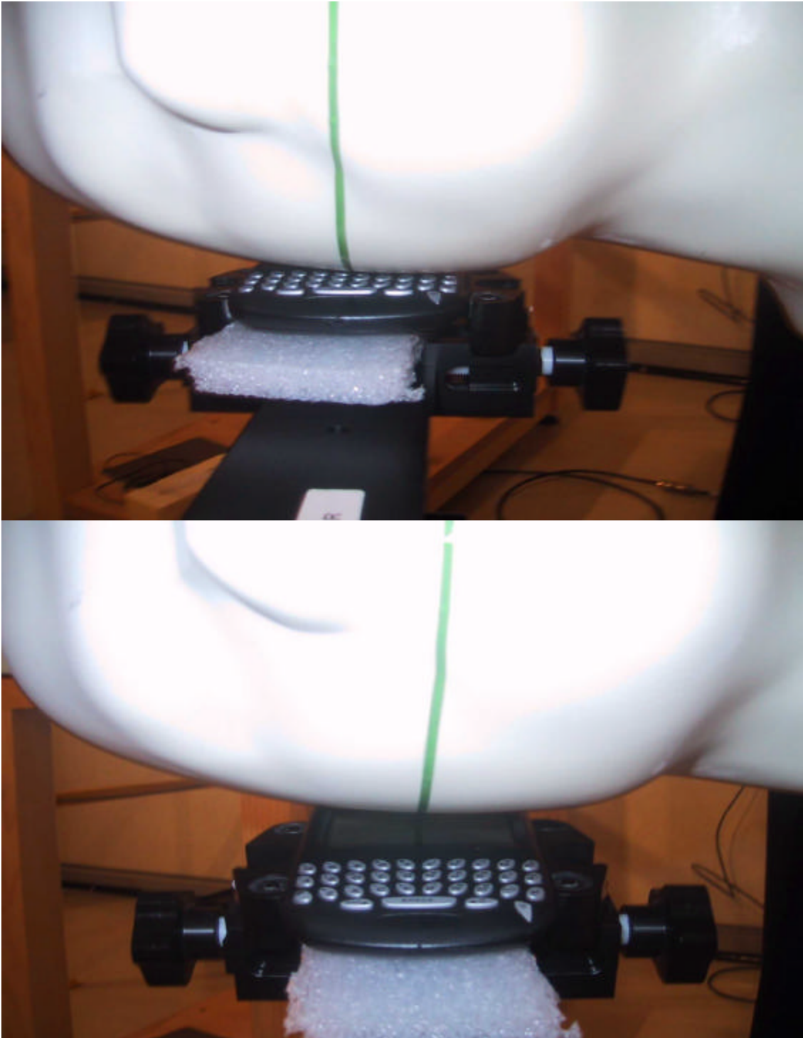
Figure B2. Right ear configuration, touch and tilted 15 degrees
