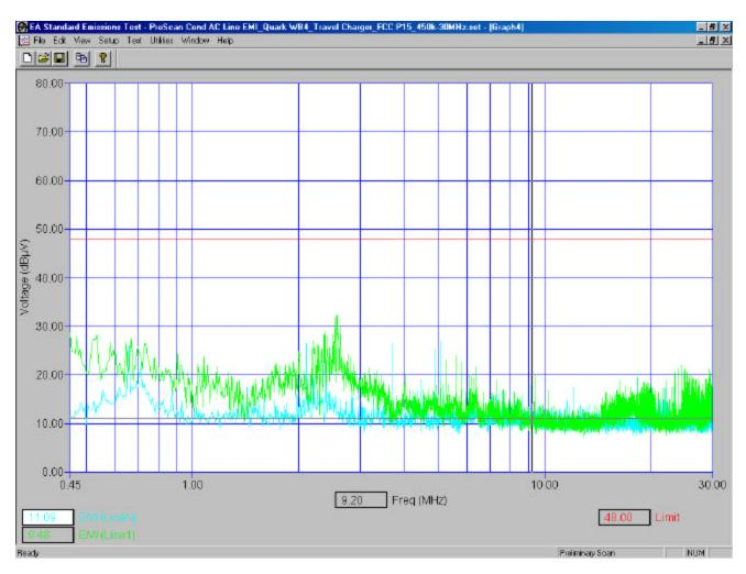
120 volt, 60 Hz ac input to ac Travel Charger, model number PSM05R-050Q, RIM part number ASY-04078-001 connected to model number R6220GW.
