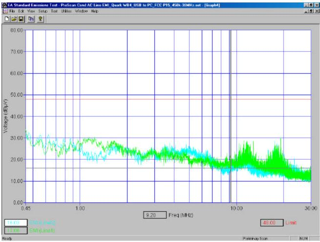
The ac input was 120 volts, 60 Hz to the support PC which was connected to the handheld via the USB data cable.
