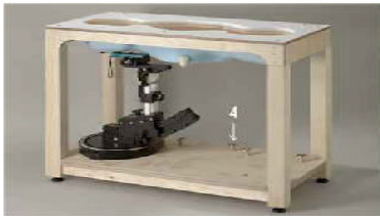
Figure 4 SAM Twin Phantom
