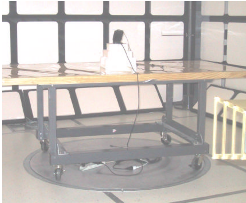
Radiated Emissions at 3.0 metres
