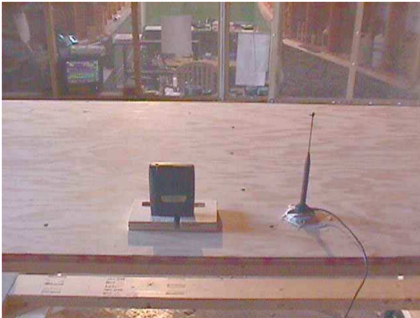
Test Configuration # 4: EUT Standalone (Upright Position)
