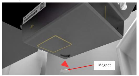
2. Place the magnet within the magnet recess on the front of the housing. Hold the magnet within the magnet ring for at least 5 seconds, then remove the magnet from the module. The module will reboot and reconnect to the previously paired Radar H2M IS module.
