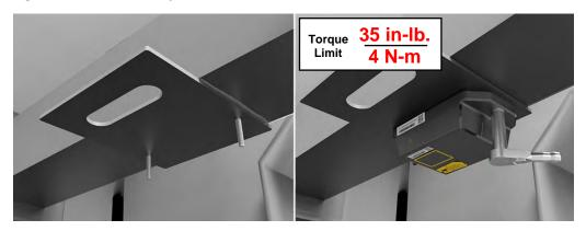
9. Once you have installed the module on the asset, create a record of the module-toasset-to-accessory pairing within the BlackBerry Installation App by recording the asset identifier and scanning the module identifier for the BlackBerry Radar R2 IS and associated Radar H2M IS module. Remove the small temporary S/N label.
