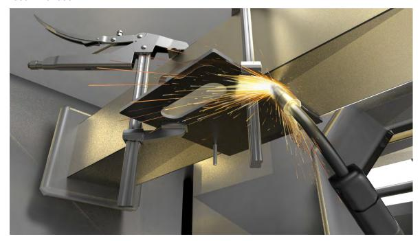
**IMPORTANT:** If you are welding the bracket to your asset; it is recommended to remove the Radar R2 IS module from the bracket before welding the bracket to the rail car. While the Radar R2 IS module can be mounted to the bracket, before the bracket is welded to the rail car, it is the responsibility of the installer to ensure the Radar R2 IS module is protected from weld splatter and extreme temperatures.
