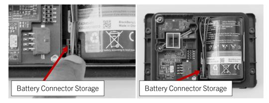
5. Place the battery cover onto the module. Place the screws in the recess on the mounting flange and cover with tape. Leaving the screws uninstalled is recommended as an indicator to the recipient that the battery is disconnected and must be connected before its next use. Module is now ready for placement into the UN certified Dangerous Goods packaging.
