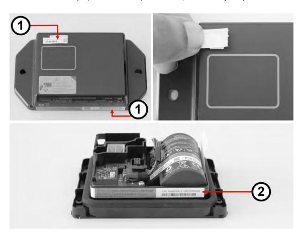
1. Once you have installed the module on the asset, create a record of the module-toasset-to-accessory pairing within the BlackBerry Installation App by recording the asset identifier and scanning the module identifier for the BlackBerry Radar R2 IS and associated Radar H2M IS module.
