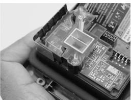
4. Fully install the battery door.
