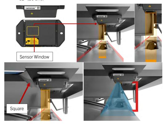
5. Once placement location is confirmed, use a pencil or marker to mark the outline of bracket for welding.
