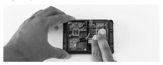
2. Connect the battery cable to the battery connector. The LED will blink to indicate the module is active. NOTE: It can take between 10-15 seconds for the blink sequence to begin. Please be patient. Once you see the LED blink, continue to the next step.
