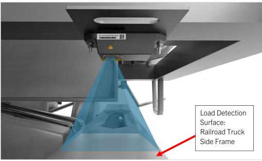
**IMPORTANT:** The orientation of the Radar R2 IS sensor module, relative to the orientation of the Load Sensor Bracket, will be determined by the installation position required by your rail car's construction and where the Radar R2 IS module and bracket assembly must be installed to monitor the railroad truck side frame. Multiple orientations are possible. Examples shown below.
