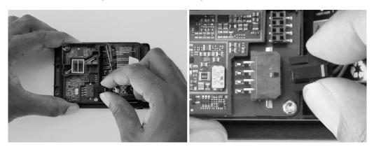
4. Store the battery cable by placing the battery cable connector in the spot below the battery. **NOTE:** Battery cable must be stowed for transit to prevent unintended contact with the battery terminals.
