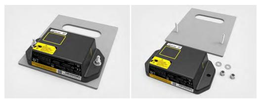
8. If you elected to remove the device while welding the bracket to your asset, ensure the bracket has cooled before re-attaching the Radar R2 IS to the to the bracket. Do not tighten the fastener beyond 35 in-lb. (4 N-m).
