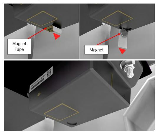
**IMPORTANT:** The magnet functions as the "Power" switch for the module. The magnet must be completely removed from the module for the module to operate.
