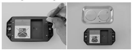
2. To separate the battery door from the outer housing—begin by inserting a flat screwdriver (3-7mm width) into a slot, marked with the arrows, and pry upwards. Complete the battery door removal by working your way around the door--inserting the screwdriver into the other slots and prying upwards, until the door is free.
