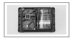
**IMPORTANT:** To transport, or ship your module with the battery, the module must be powered off. If the battery is disconnected, there is no power to the device and the device is powered off.
