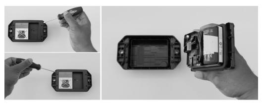
3. Disconnect the battery cable from the battery connector.
