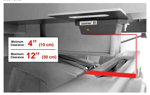
**IMPORTANT:** For accurate load detection, it is important to ensure there is a **minimum** clearance of 4" (10 cm) between the sensing surface of the module and the top surface of the axle.
