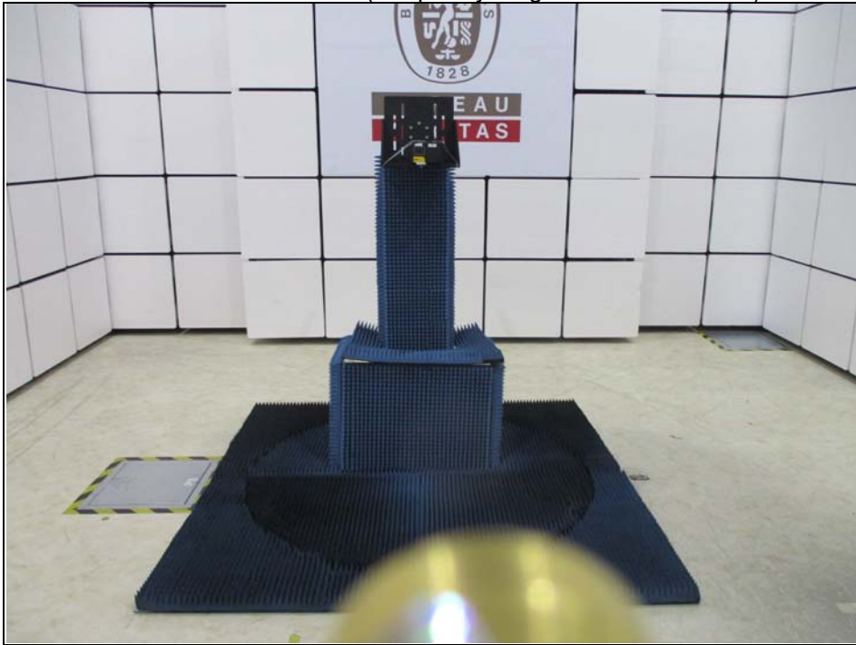
Radiated Emission Test (Frequency range 110GHz ~ 170GHz)
