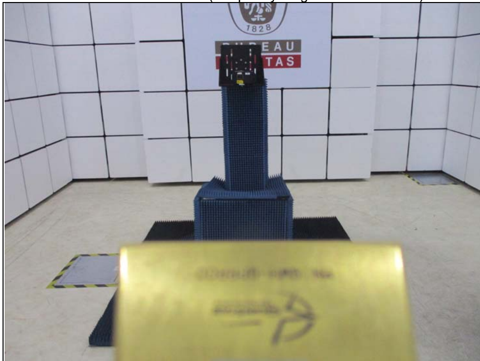
Radiated Emission Test (Frequency range 50GHz ~ 75GHz)
