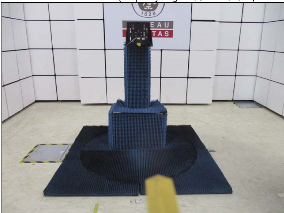
Radiated Emission Test (Frequency range 220GHz ~ 231GHz)
