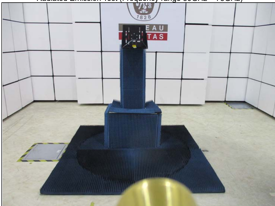
Radiated Emission Test (Frequency range 50GHz ~ 75GHz)
