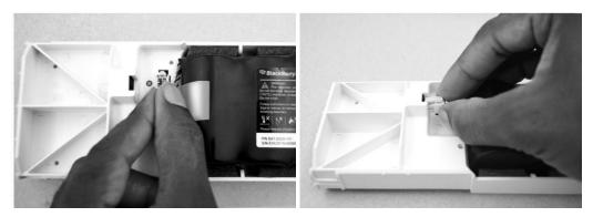
3. Remove the battery from the battery compartment by grasping the pull tab and lifting the battery out of the compartment.
