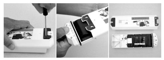
2. Ensure the battery cable is disconnected from the battery connector. Place the battery cable in the battery connector nest.
