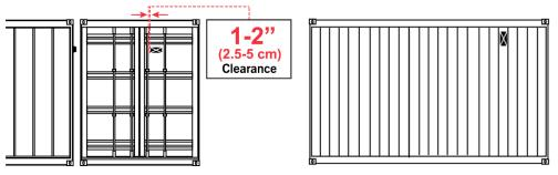
**IMPORTANT:** If you intend to pair your BlackBerry Radar H2 module with a BlackBerry Radar Cargo Accessory, please ensure you do not install the BlackBerry Radar H2 module at a height that prevents the installation of the Cargo Accessory at the required placement heights in the illustration, below.
