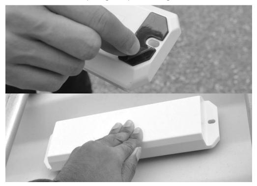
6. Insert your fastener of choice into the holes and use the appropriate tools to secure the module to the asset.
