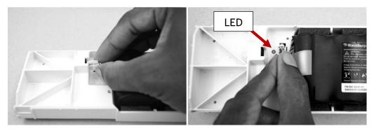
4. Completely insert the inner housing into the outer housing.
