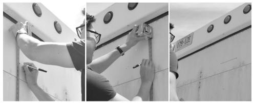
4. Remove the adhesive from the rear of the template and place the template in the desired installation location. The adhesive at the back of the template ensures that it stays on the door surface for accurate drilling of your holes.
