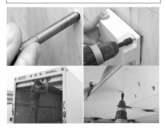
6. Remove the template. You now have four holes in the door. If there are any burrs around the holes, remove them at this time. Also, remove any dust or debris left over from the drilling or de-burring operations.
