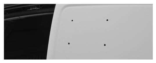
2. Source a set of nylon or rubber plugs, of the appropriate diameter, to fill the holes. These plugs can be sourced from hardware or auto supply stores. Insert the plugs into the holes. If desired, you may add 100% Silicone Exterior Grade caulk to the rear of the plug for extra protection to seal any gaps against water entry.
