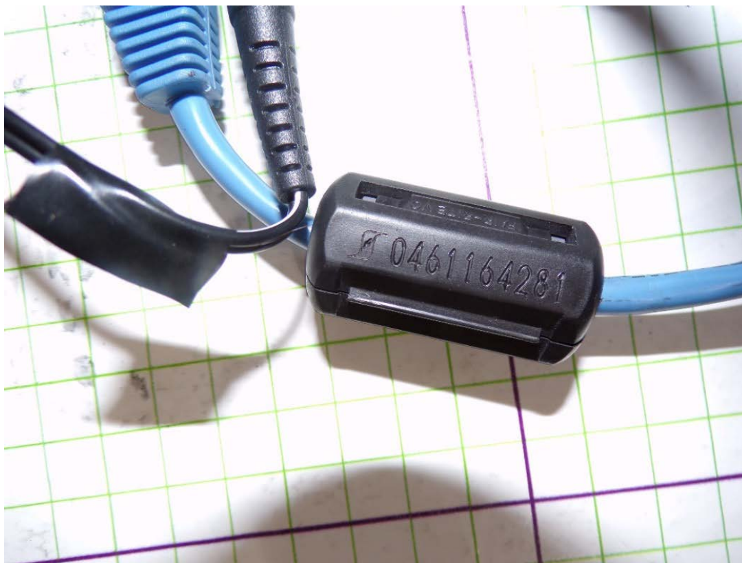
Radiated Emissions Ferrite Modification on Ethernet Cable
