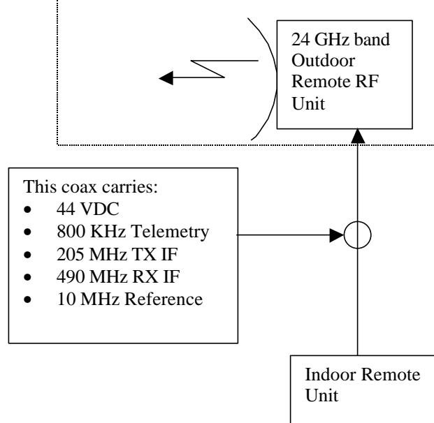
Within the Point to Multipoint network the Hub will support Multiple Remote Units. The Hub antenna will have up to 90 degrees of azimuth coverage. Exhibit N of each application contains information about the antennas.
