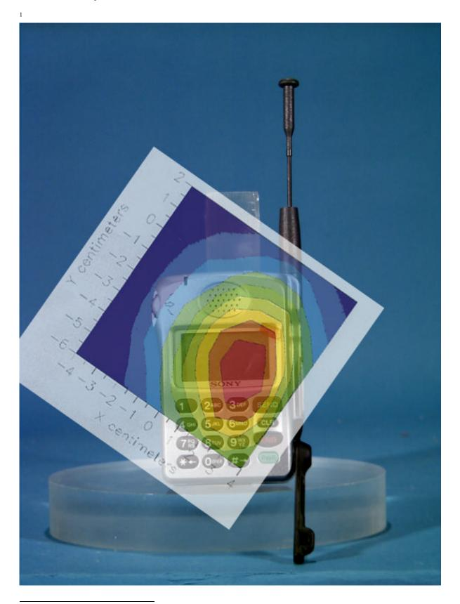
$<sup>^{1}</sup>$  Peak SAR Value at the surface of the phantom @ Z = 0 (not averaged over 1-gram of tissue). This is a computer simulation of the hot spot(s) of the phone.
