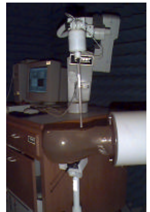
Fig. 1 SAR Test Set-up
