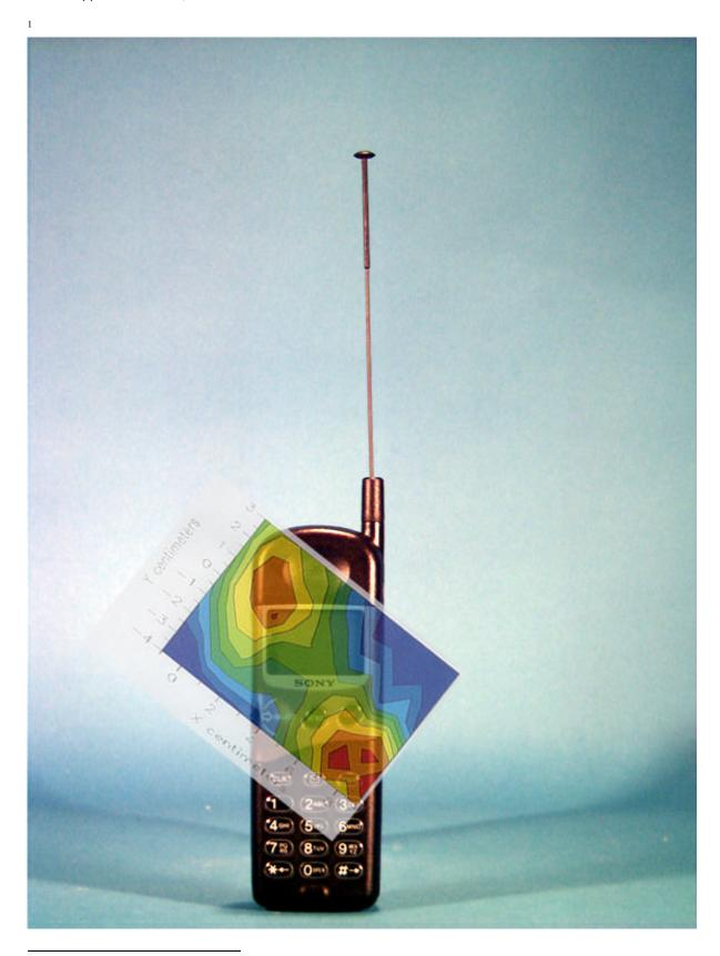
$<sup>^1</sup>$  Peak SAR Value at the surface of the phantom @ Z=0 (not averaged over 1-gram of tissue). This is a computer simulation of the hot spot(s) of the phone.
