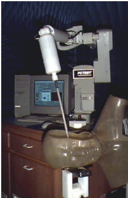
Figure 5. Photograph of the Probe and the Phantom
