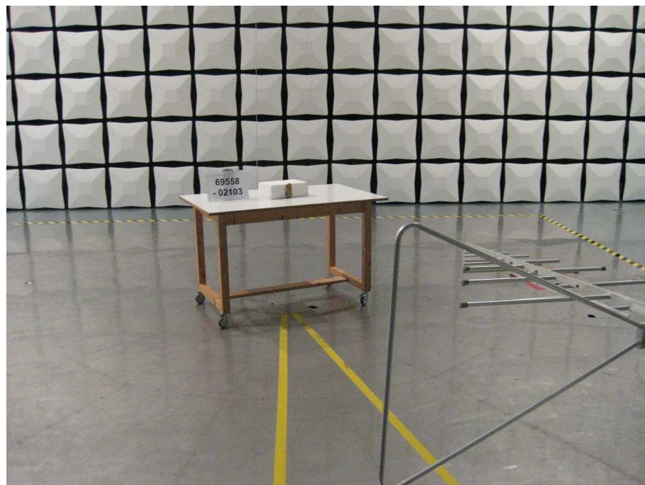
**Test setup for radiated emission measurement
