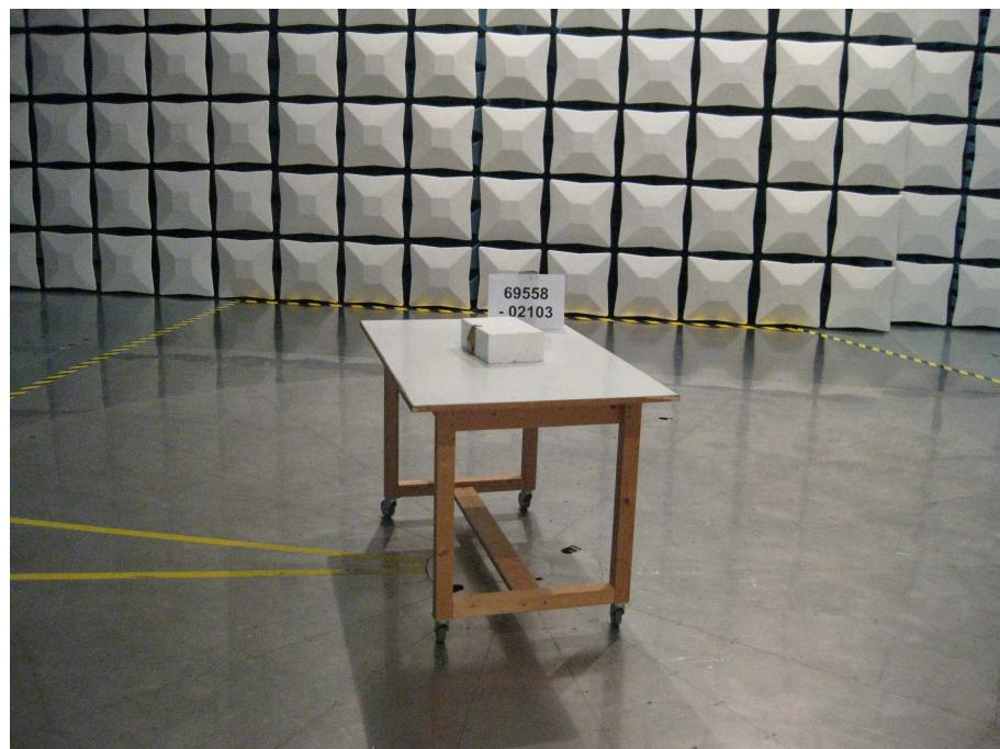
**Test setup for radiated emission measurement
