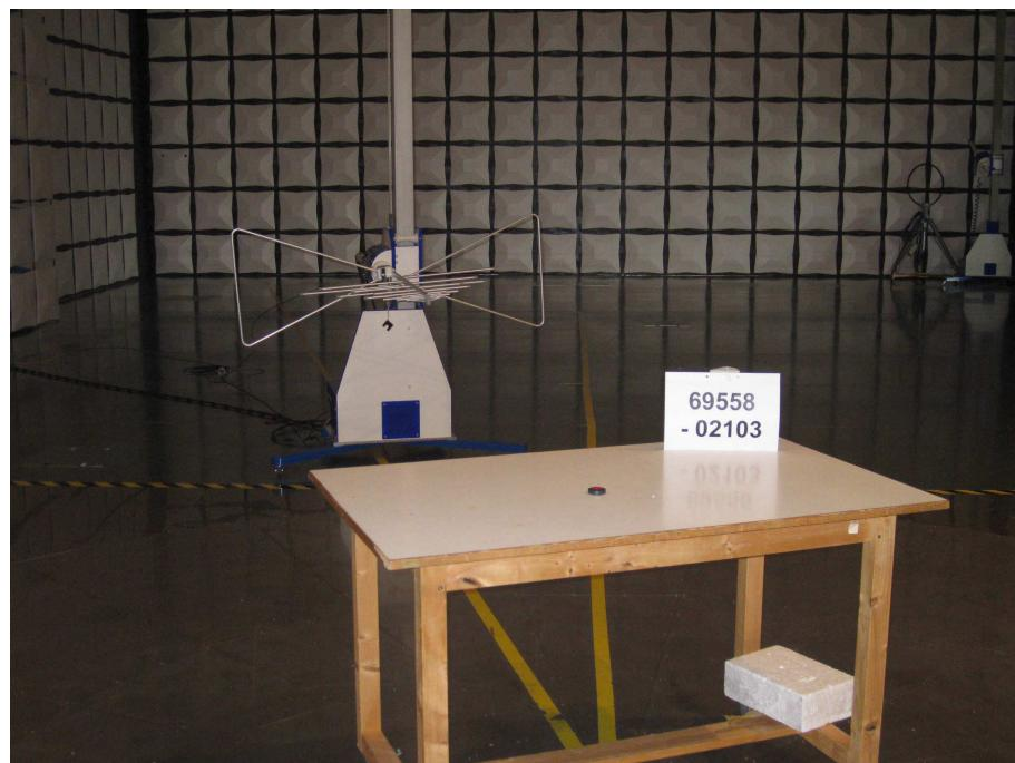
**Test setup for radiated emission measurement
