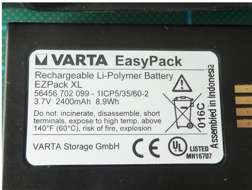
170685EUTexternal: Battery type plate
