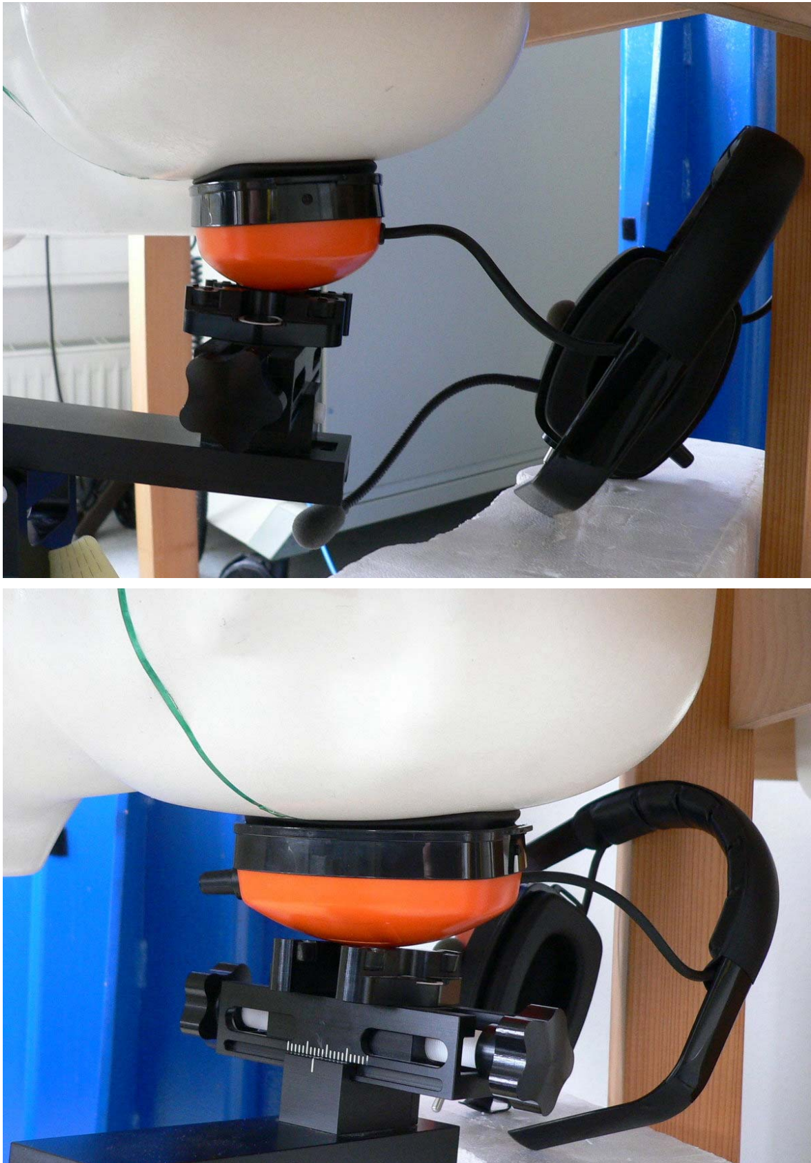
Fig. 13: Cheek position, left side (left earpiece).
