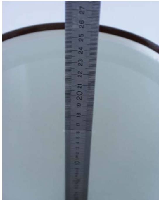
Fig. 15: Liquid depth for the US DECT Head measurements.
