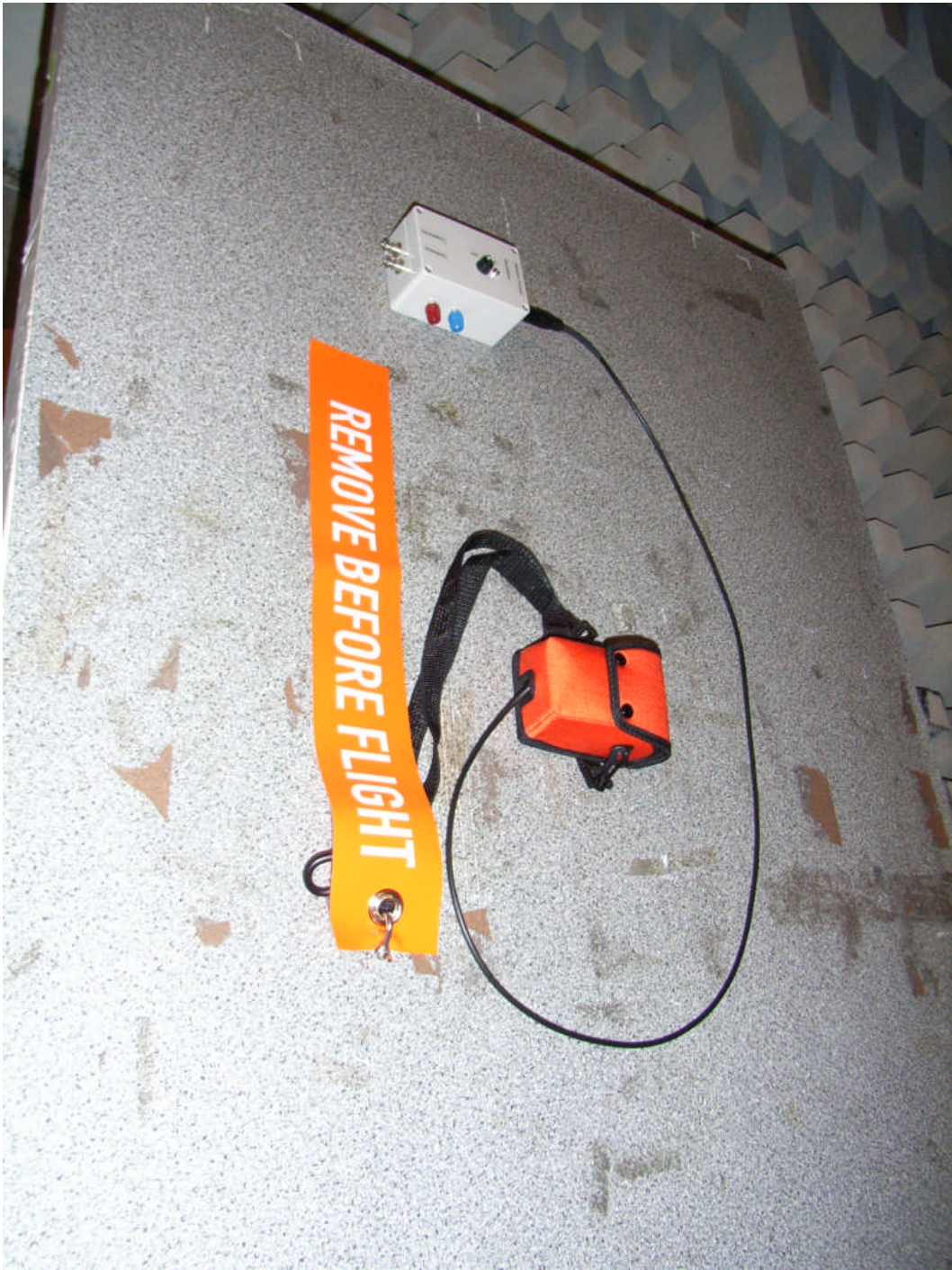
80535_EMI2.jpg Test set-up radiated emission test
