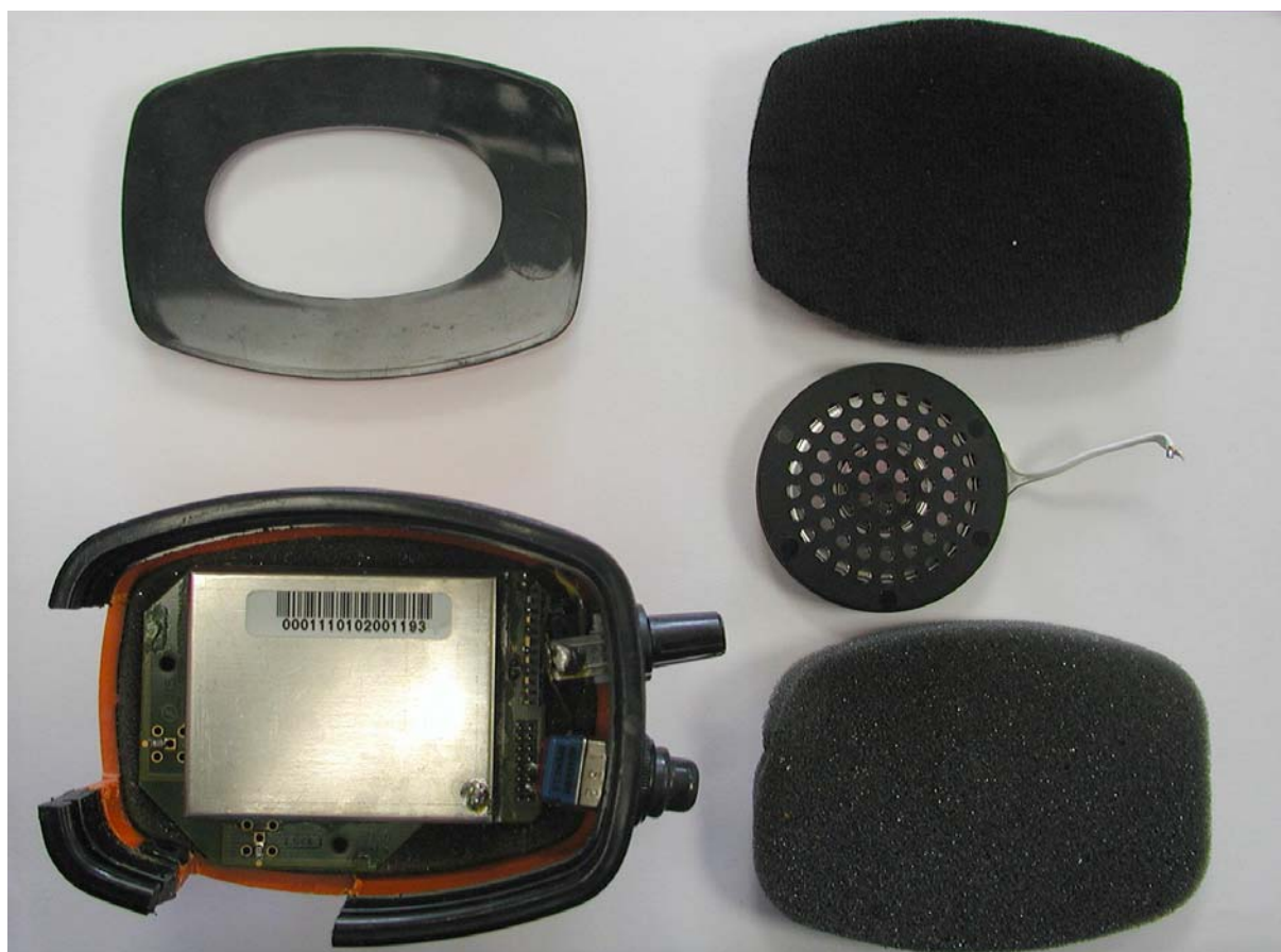
Photo 7 : CT-DECT-H24 / Disassembled headset
