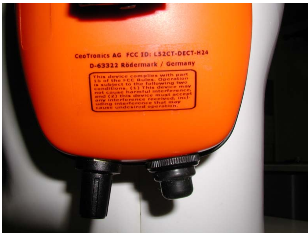
Photo 4: CT-DECT-H24 Headset Left Side View and External Labeling
