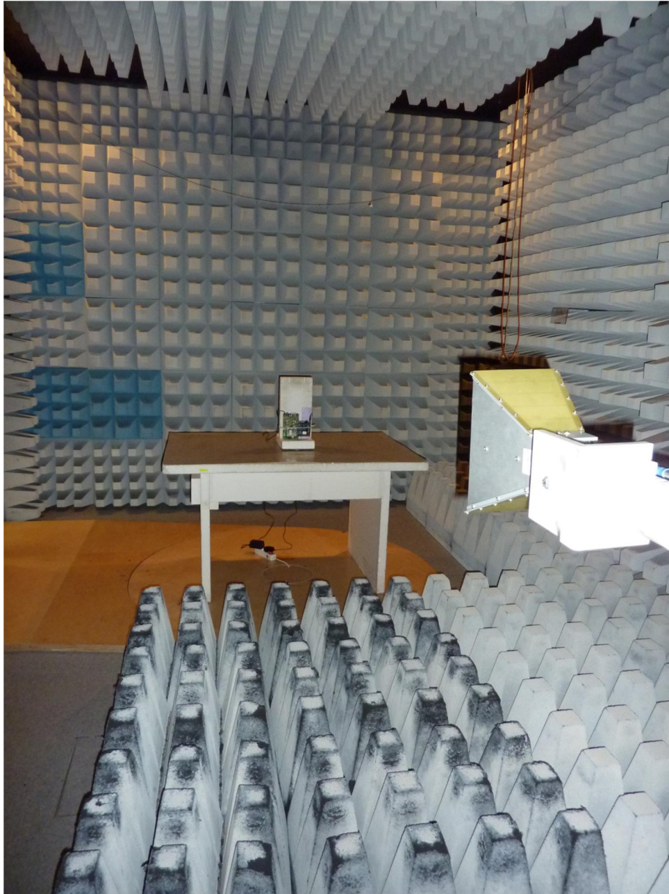
134429_2.JPG: Test setup fully anechoic chamber
