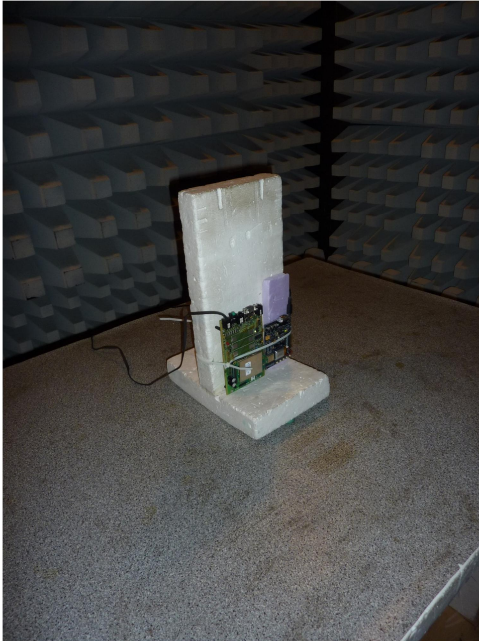
134429_5.JPG: Test setup fully anechoic chamber
