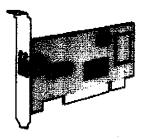
This Fast Ethernet PC ladapter is a dual-speed adapter connected to an Ethernet network with a single connection over Unshielded Twisted-Pair (UTP) cable. The adapter automatically senses and switches to either 10 Mbps or 100 Mbps. For 100 Mbps operation, the adapter supports operation on Category 5 UTP cable. For 10 Mbps operation, the adapter supports on Category 3, 4, or 5 UTP cable.
