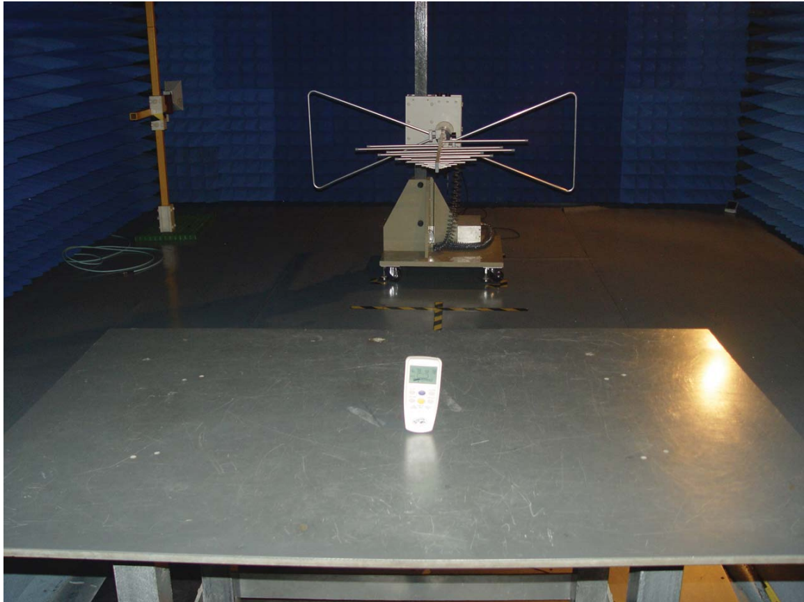
Radiated emissions test < 1GHz
