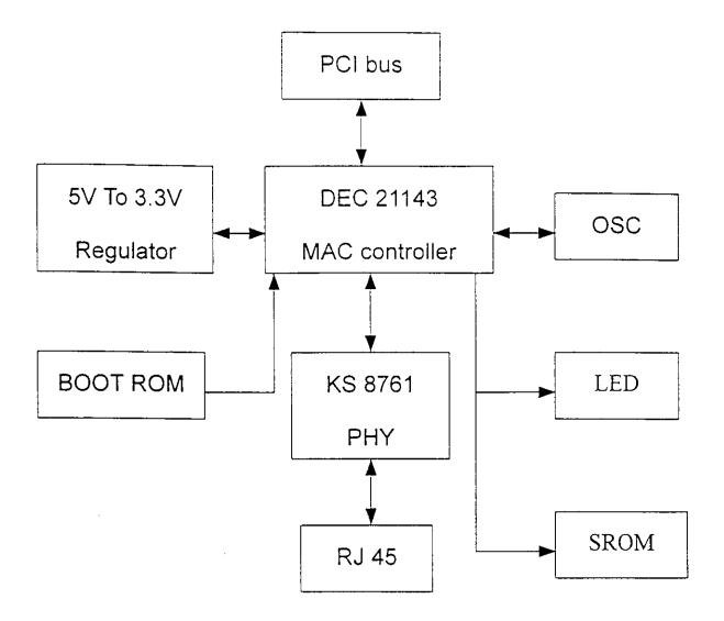
DEC 21143 : 10/100 Mbps Ethernet MAC controller supports the peripheral Component Interconnect.
