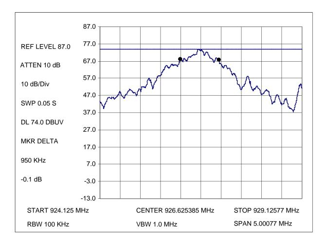
Figure 3.1 – 3 : Emission Bandwidth Plot (high channel)
