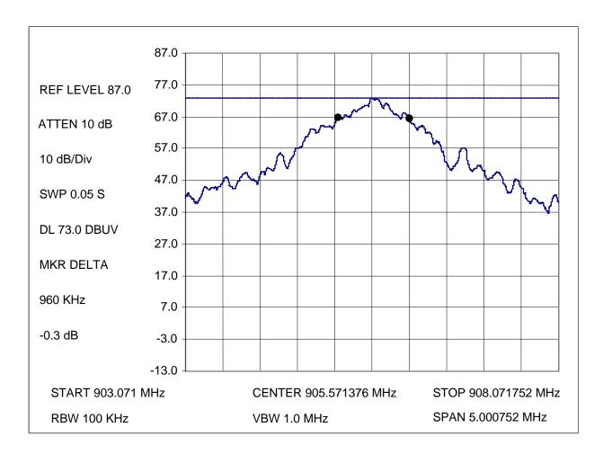
Figure 3.1 - 1: Emission Bandwidth Plot (low channel)
