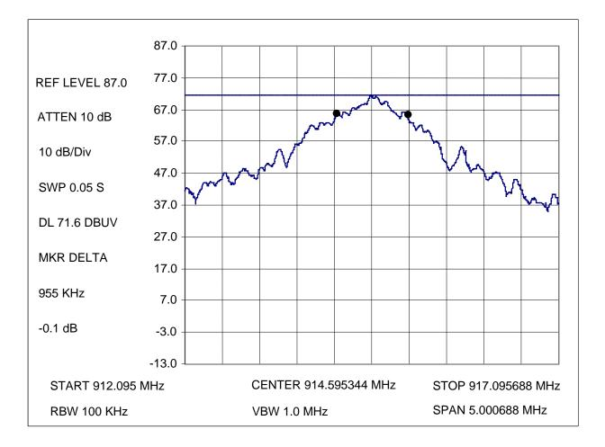
Figure 3.1 - 2: Emission Bandwidth Plot (mid channel)
