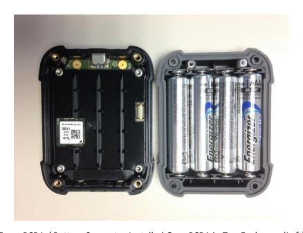
Trace PCBA / Battery Separator Installed Over PCBA in Top Enclosure (Left)
