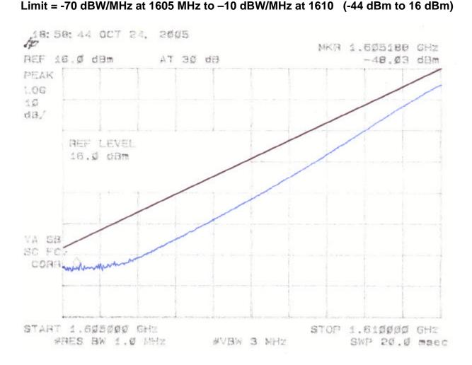
Measured Value is -48.03 + 0.25 (cable loss) = -47.78
