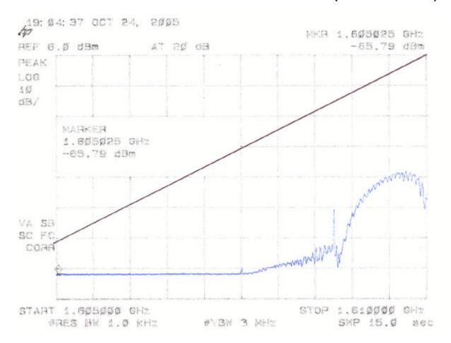
Measured Value is -65.79 + 0.25 (cable loss) = -65.54 dBm
