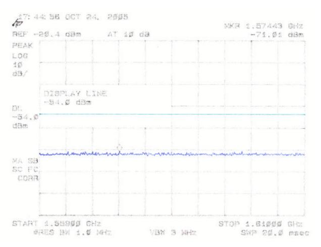
Measured Value is -71.01 + 0.25 (cable loss) = -70.76 dBm
