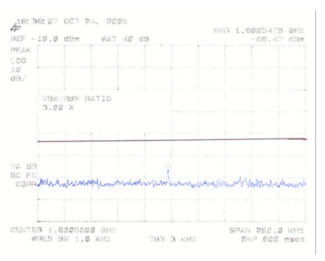
Measured Value is -66.47 + 0.25 (cable loss) = -66.22
