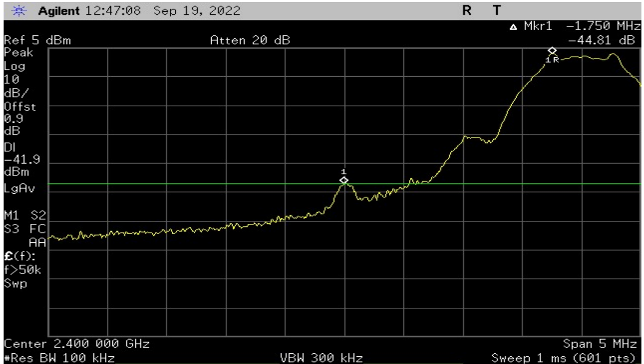
Plot 21 - Band Edge – Low Channel
