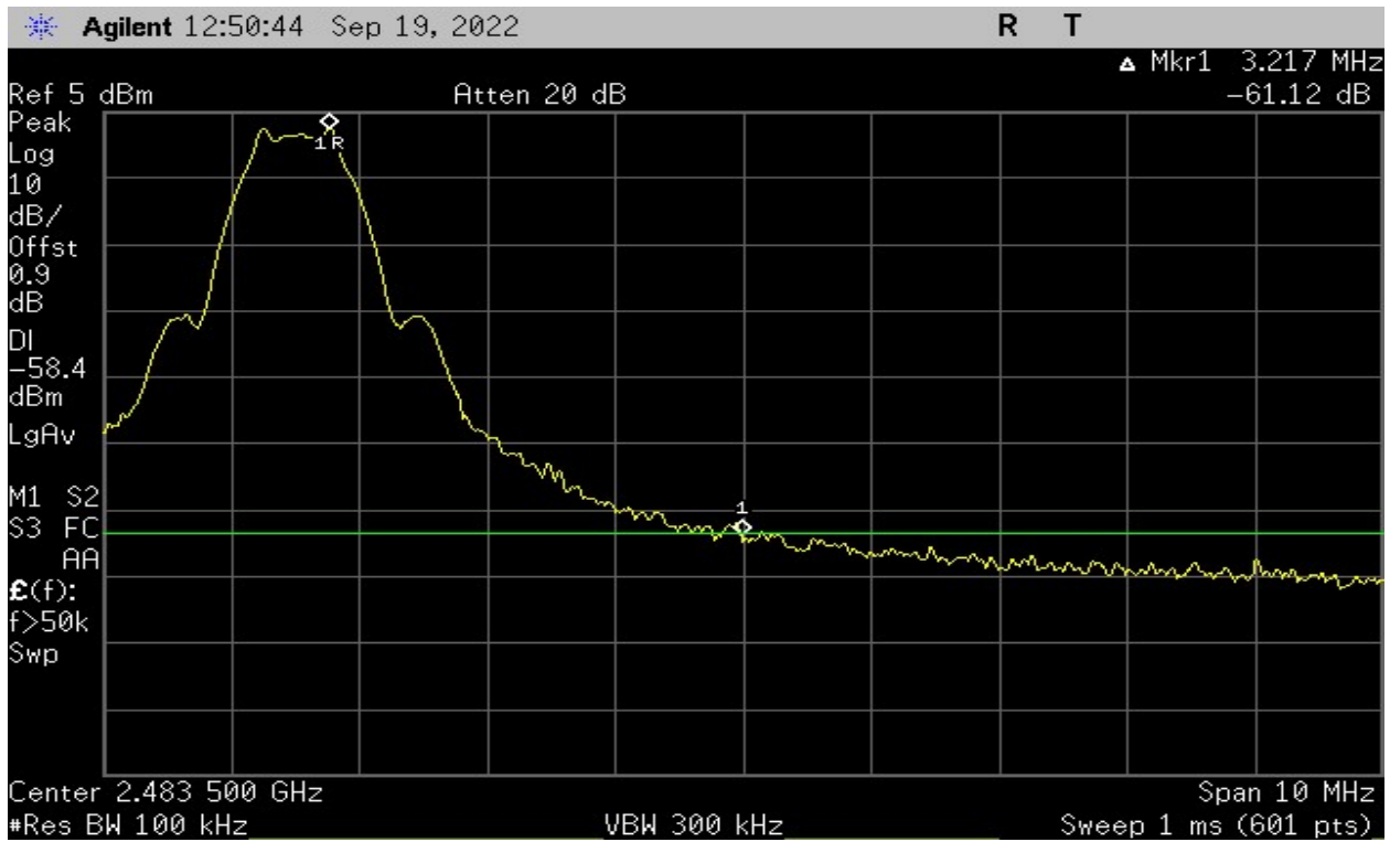
Plot 22 – Band Edge - High Channel
