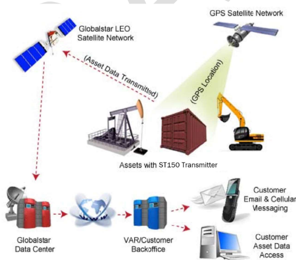
FIGURE 3 - SIMPLEX IoT MESSAGING Data Flow
