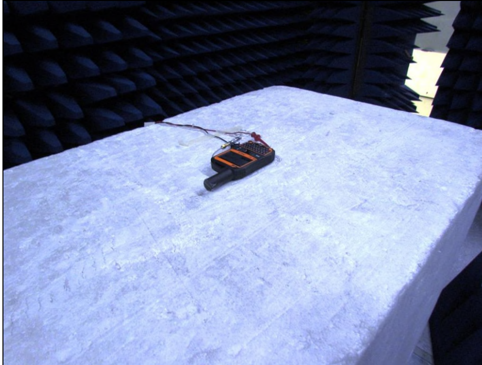
Figure 6: Equipment Under Test – Radiated Emissions – Y-orientation
