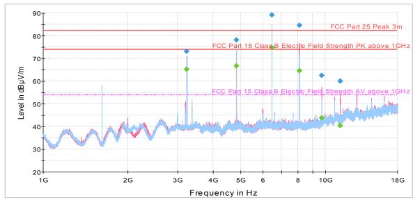
FCC Part 15 Class B Electric Field Strength PK above 1GHz [..\EMI Radiated\] FCC Part 15 Class B Electric Field Strength AV above 1GHz [..\EMI Radiated\]
