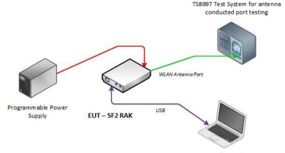
Support Laptop for configuring RF functions of the EUT
