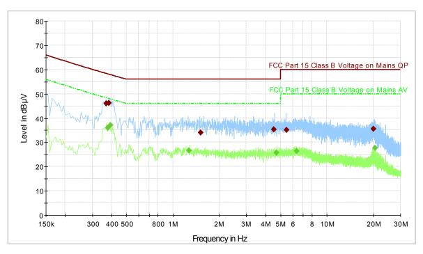
FCC Part 15 Class B Voltage on Mains QP [..\EMI conducted\] FCC Part 15 Class B Voltage on Mains AV [..\EMI conducted\]
