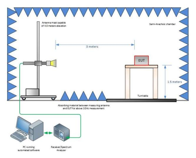
Radiated Emission Test Setup (Above 1GHz)
