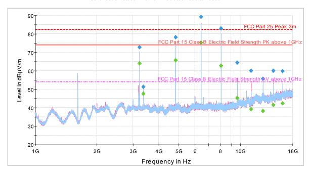
FCC Part 15 Class B Electric Field Strength PK above 1GHz [..\EMI Radiated\] FCC Part 15 Class B Electric Field Strength AV above 1GHz [..\EMI Radiated\]
