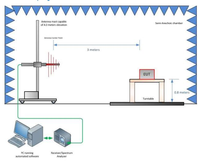
Radiated Emission Test Setup (Below 1GHz)
