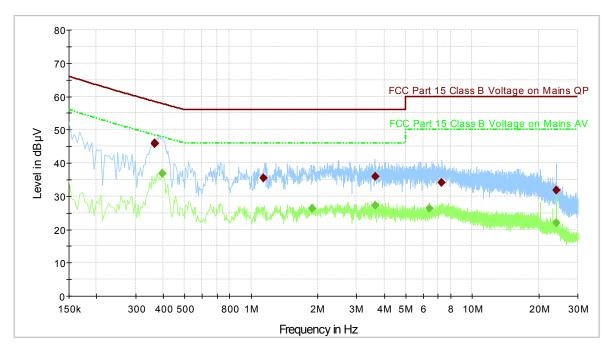
FCC Part 15 Class B Voltage on Mains QP [..\EMI conducted\] FCC Part 15 Class B Voltage on Mains AV [..\EMI conducted\]
