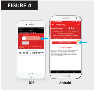
**NOTE:** The Sat-Fi2 will remain in S.O.S. mode until cancelled by the user. The S.O.S. notification to GEOS will not be cancelled if the device is powered off or if the Sat-Fi2 App is turned off.
