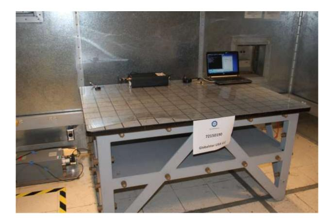
AC Conducted Emissions Test Setup
