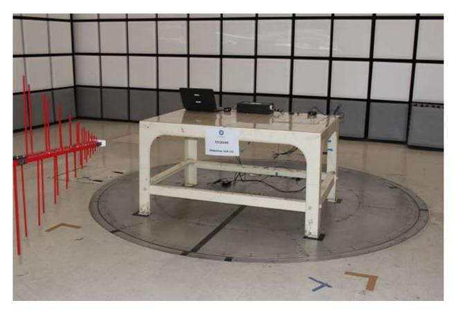
Radiated Emissions Test Setup (below 1GHz)
