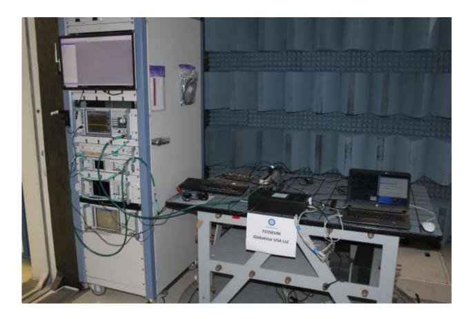
Antenna Conducted Port Test Setup
