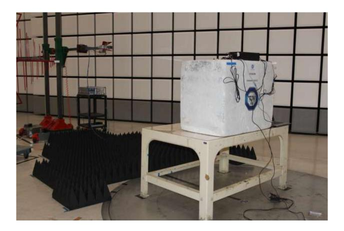
Radiated Emissions Test Setup (Above 1GHz)
