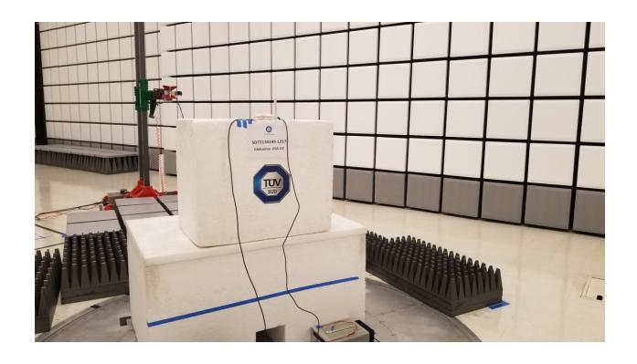
Radiated Emissions Test Setup (above 1GHz)
