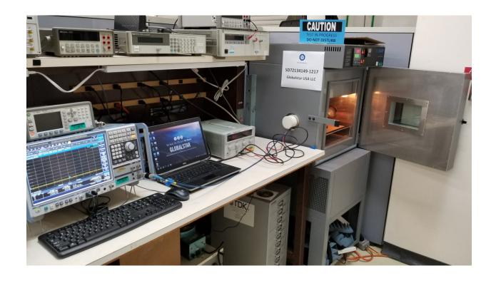
Frequency Stability/Voltage Variation Test Setup
