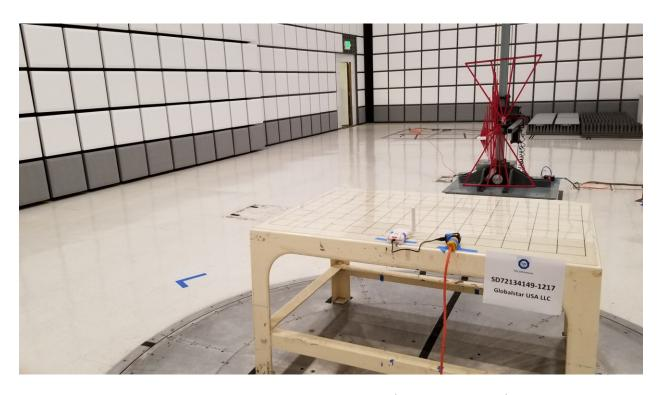
Radiated Emissions Test Setup (below 30MHz)
