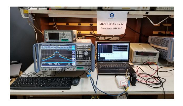
**Conducted Antenna Port Test Setup (Satellite)**
