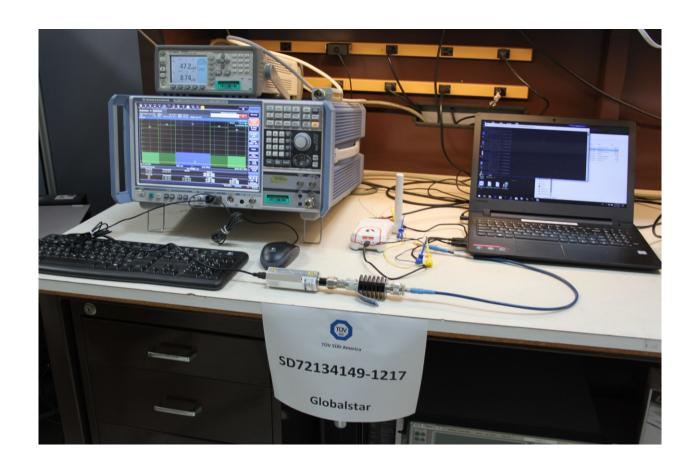
**Conducted Antenna Port Test Setup (WLAN)**
