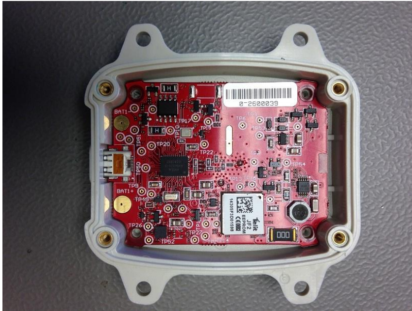
PCB Installed in Bottom housing (Battery plate Removed)
