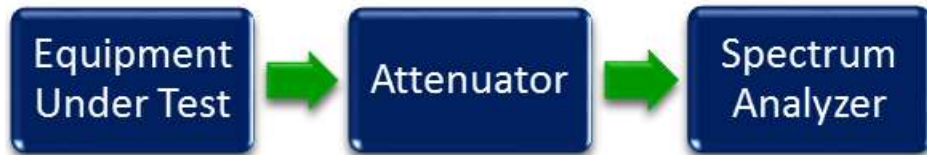
Figure 4. Conducted Spurious Emissions Test Setup
