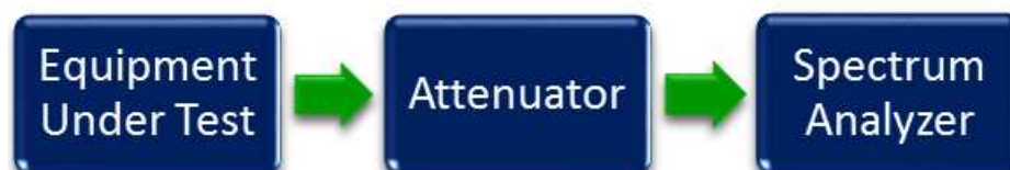
Figure 6. Band Edge Test Setup
