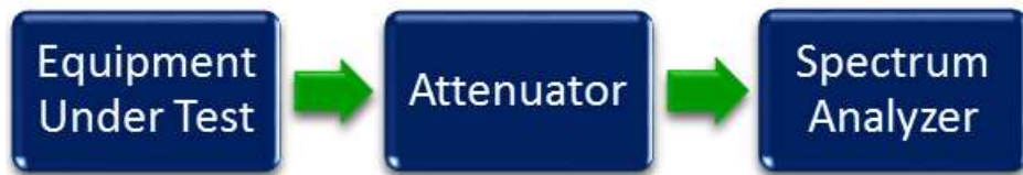
Figure 3. RF Power Test Setup
