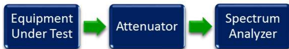
Figure 2. Occupied Bandwidth Test Setup
