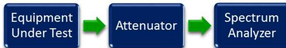
Figure 2: Spurious Emission at Antenna Terminal Test setup
