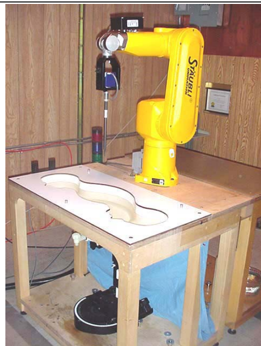
DASY4 System with SAM Phantom and device holder
