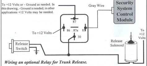
CONNECTION: An optional relay is required. Connect the Gray wire to relay pin 85, and connect +12 Volts to relay pin 86. Connect pins 87, 87a & 30 as indicated in the diagram.
