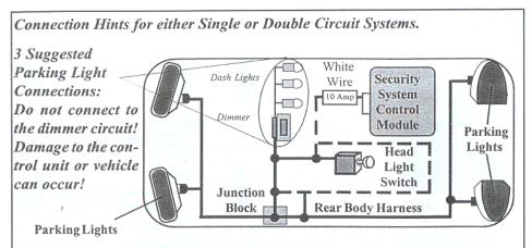
Red/White Wire - (+ or - Flashing Light Input): This wire supplies + 12 Volt or - Ground to the White wires for when the system flashes the parking lights. This wire is pre-connected to +12 Volts in the main wiring harness- if connection to - Ground is needed, cut and connect as needed.
