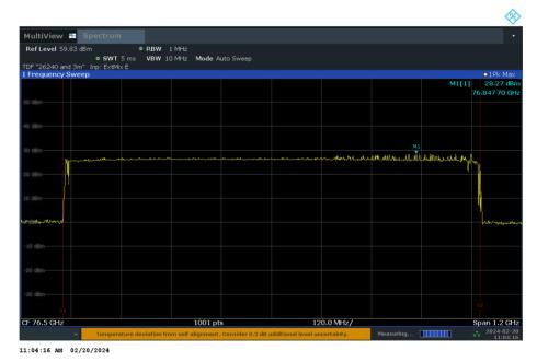
Operating mode - Continuously Transmitting - 12.0 V DC power supply
