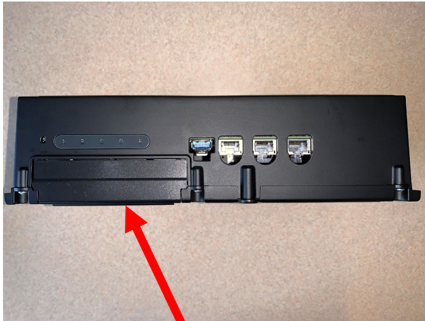
Plastic cover installed
