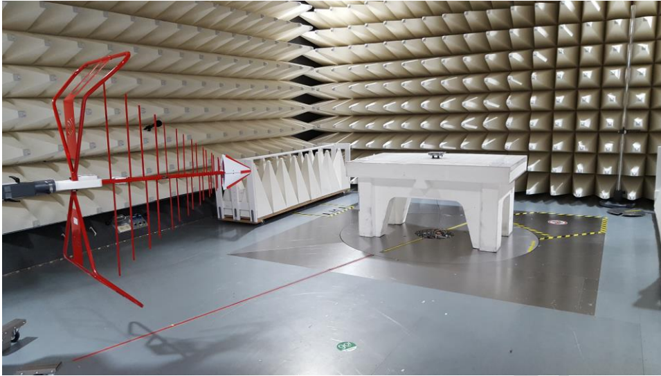
Figure B5. Low Range Radiated Emission test setup (30MHz to 1GHz)
