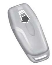
1. Slide the release on the back of the remote control and pivot the cover off.
