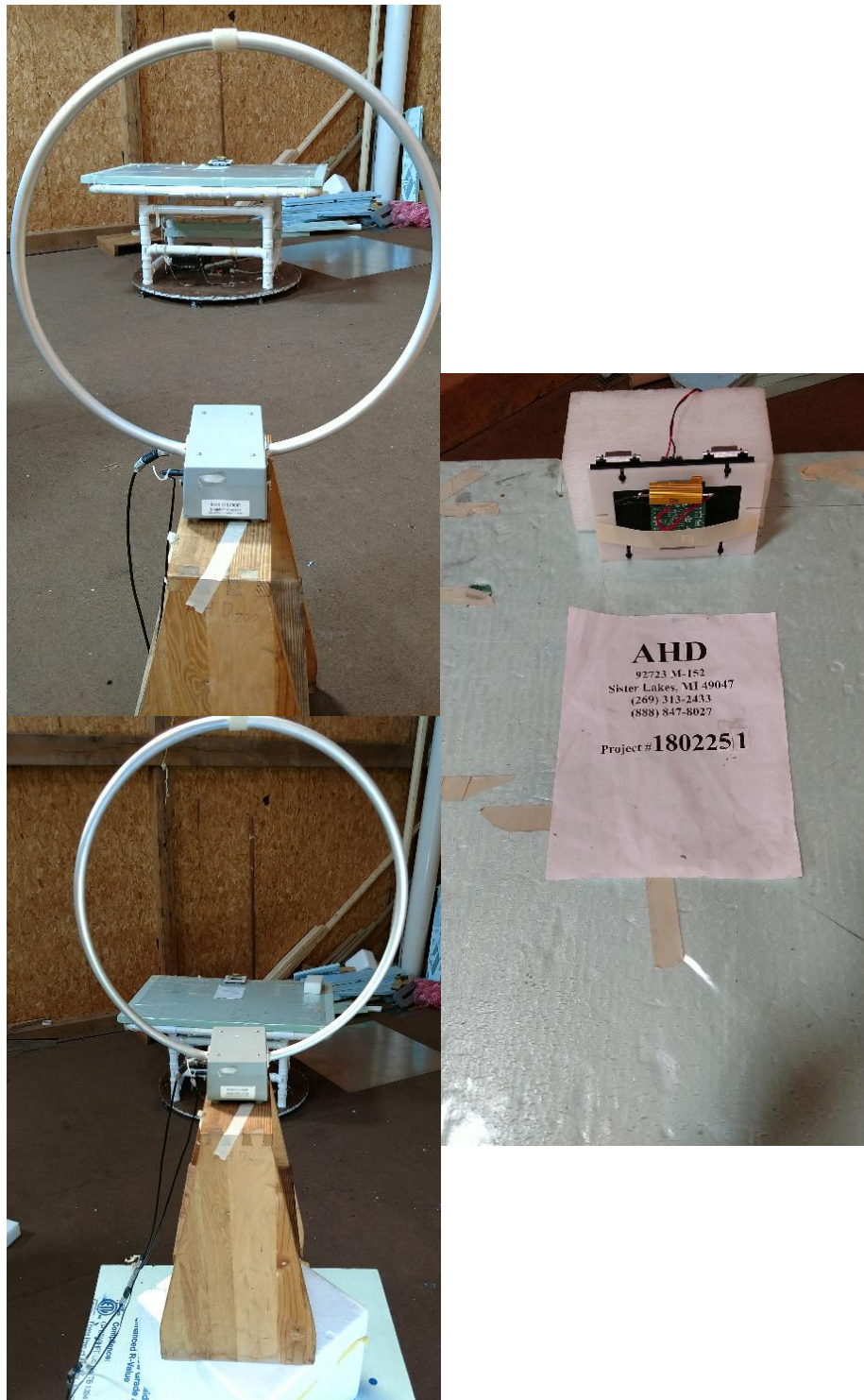
Figure 4: Radiated Emissions Test Setup Photograph(s).
