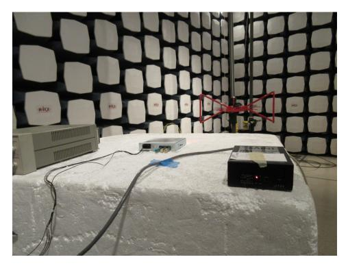
1.1 Field Strength of Spurious Radiation below 1 GHz Front View
