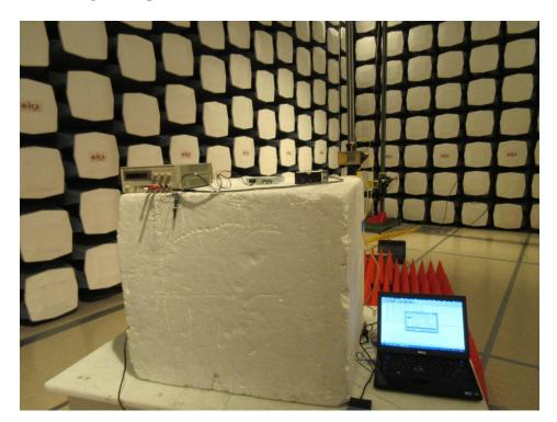
**1.3** Field Strength of Spurious Radiation above 1 GHz Front View
