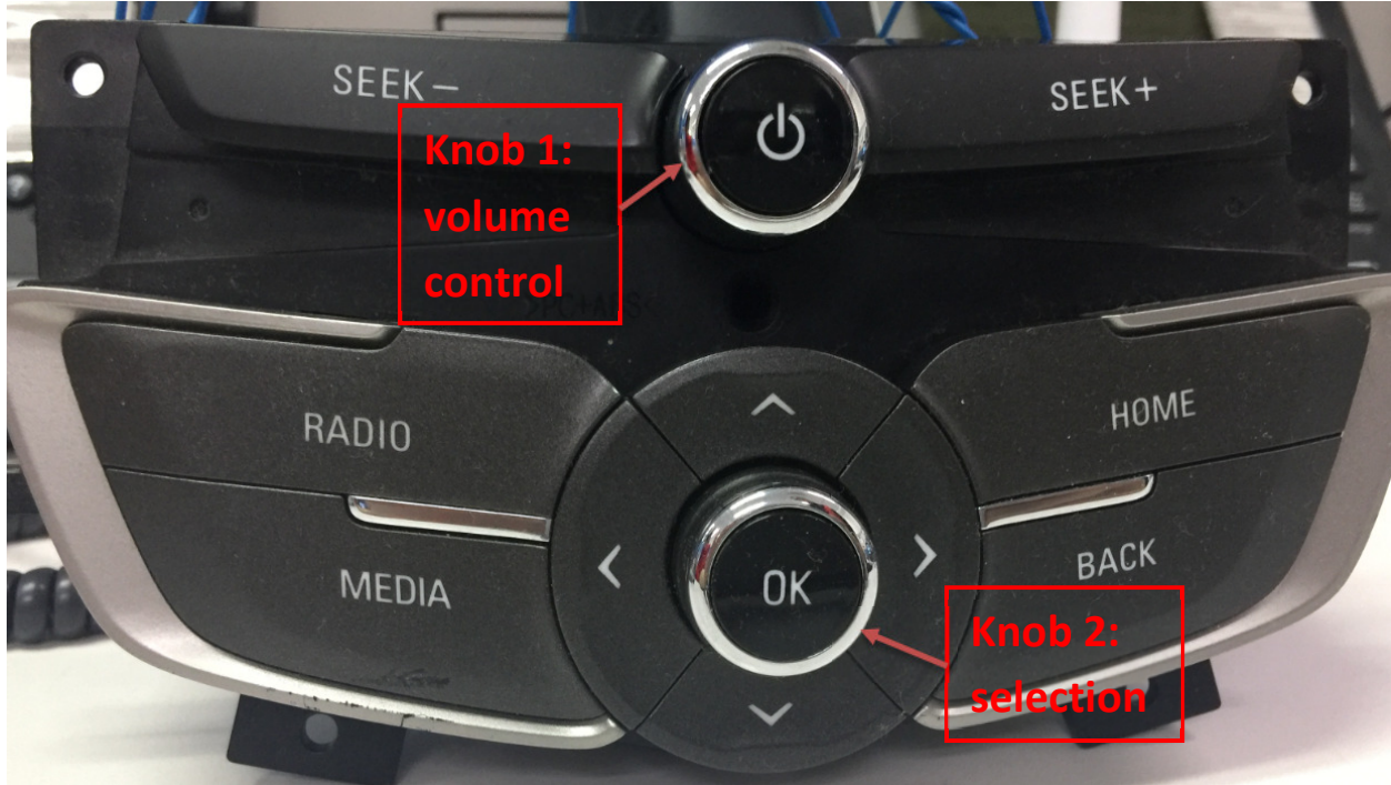
Fig. 1 Integrated Control Panel
